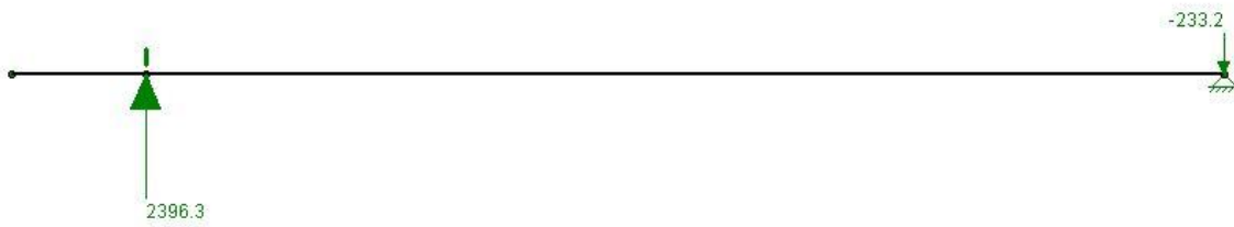
Figure 59: Plate Girder Reactions
